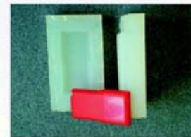
Reper realizat prin tehnologie MCP-Vacuum Casting
